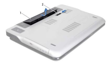
1 battery 2 battery release latch
