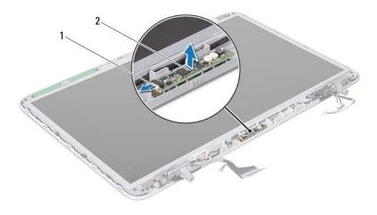
1 IR emitter board cable 2 IR emitter board
